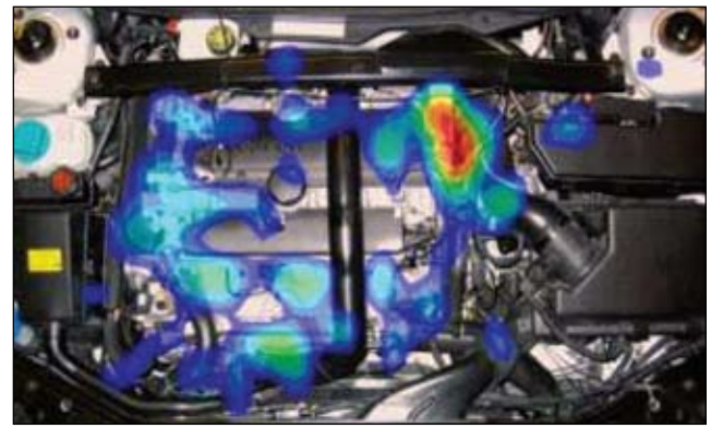
Figure 11. Noise source identification color map.
