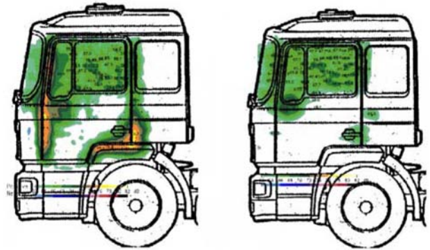
Figure 10. Acoustic beamforming results for a door seal investigation. Baseline (left) and after modifications (right)
