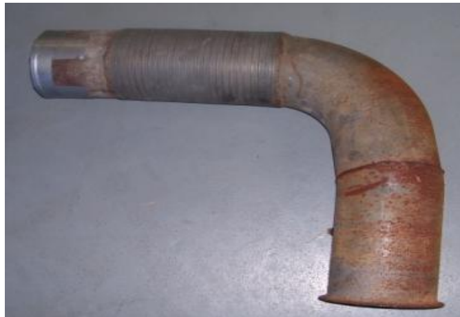
Figure 9: 84 cm \frac{1}{4} wavelength tuner designed to cancel a 102 Hz acoustic wave.
