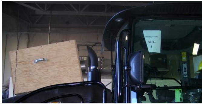
Figure 3: Artificial acoustic excitation used to excite the cab response.
